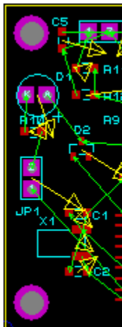
Mounting holes placed
